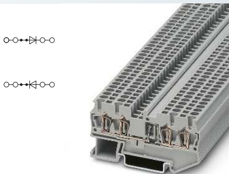
2.5 (4) mm 2 , 0.5 A, diode terminal block, 4 connections
