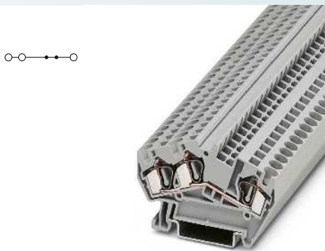
4 (6) mm 2 , 38 A, feed-through terminal block, 3 connections
