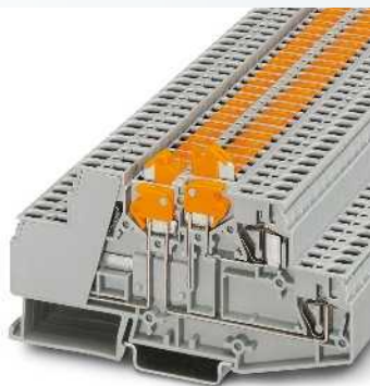
2.5 (4) mm 2 , 16 A, double-level terminal block with one disconnect knife per level
