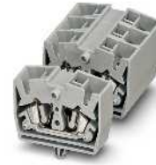
2.5 (4) mm 2 , 30 A, feed-through terminal block, 4 connections, with engagement pin
