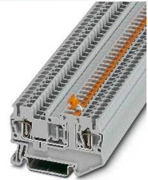
2.5 (4) mm 2 , 20 A, knife disconnect terminal block
