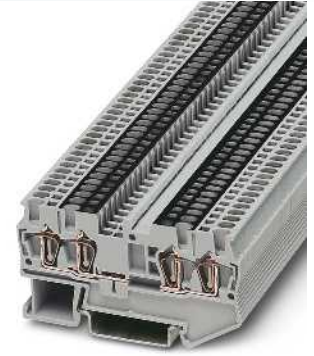
1.5 (1.5) mm 2 , 17.5 A, feed-through terminal block, 4 connections, with split power rail
