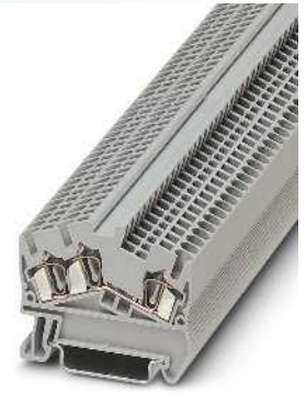
2.5 (4) mm 2 , 28 A, feed-through terminal block, 3 connections
