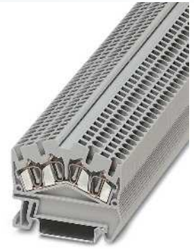
2.5 (4) mm 2 , 28 A, feed-through terminal block, 4 connections
