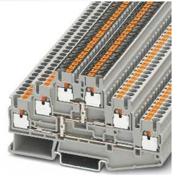
2.5 (4) mm 2 , 24 A, three-level terminal block, internally connected levels
