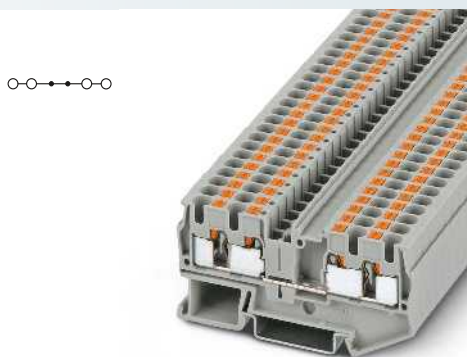
4 (6) mm 2 , 38 A, feed-through terminal block, 4 connections
