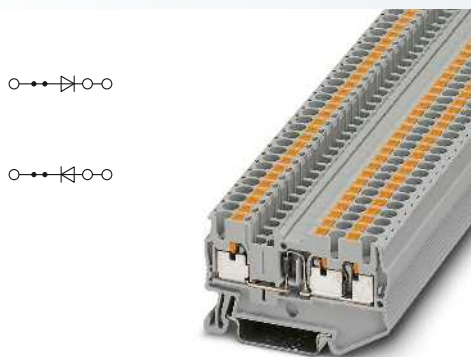
2.5 (4) mm 2 , 0.5 A, diode terminal block, 3 connections
