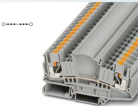
6 (10) mm 2 , 41 A, feed-through terminal block, same shape
