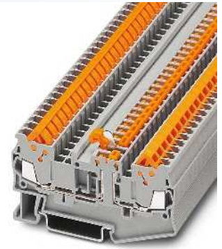
1.5 (1.5) mm 2 , 17.5 A, knife disconnect terminal block
